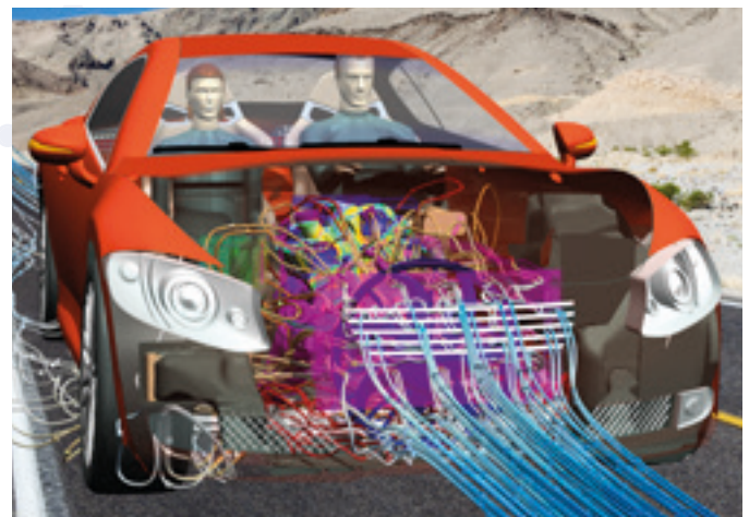
Streamlines through an engine compartment (Courtesy of InDesA GmbH)
